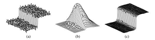
Figure 1: (a) A 100-gray-level step perturbed by Gaussian noise with  $\sigma=10$  gray levels. (b) Combined similarity weights  $c(\xi,\mathbf{x})s(\mathbf{f}(\xi),\mathbf{f}(\mathbf{x}))$  for a  $23\times23$  neighborhood centered two pixels to the right of the step in (a). The range component effectively suppresses the pixels on the dark side. (c) The step in (a) after bilateral filtering with  $\sigma_r=50$  gray levels and  $\sigma_d=5$  pixels.
