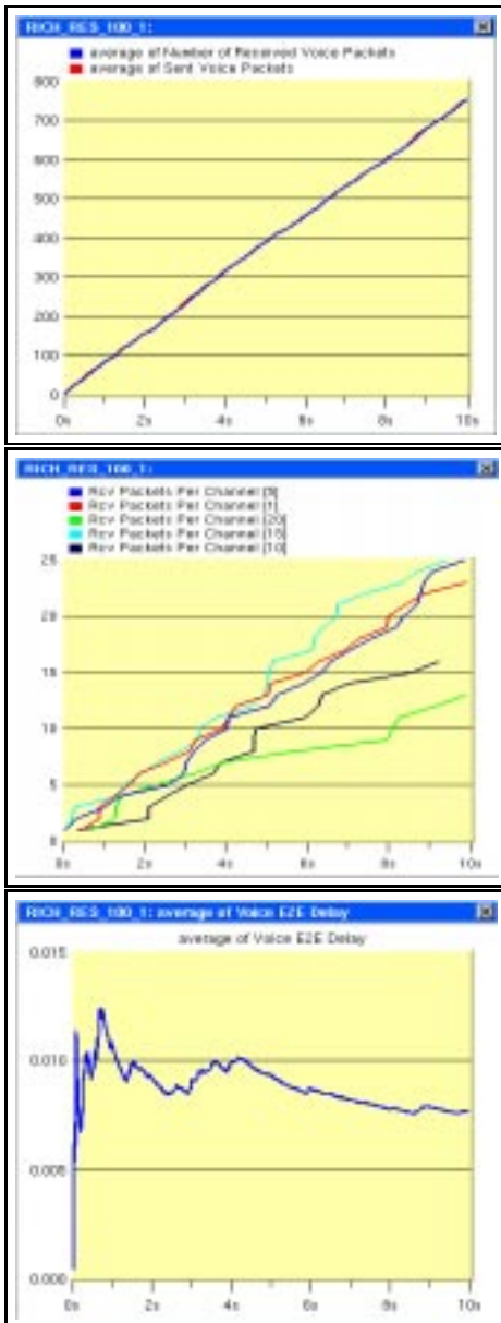
Fig. 5. Packets send with an aggregate node data rate less than the available channel bandwidth
