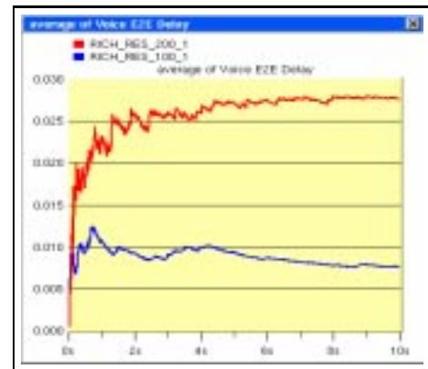
Fig. 7. Difference between an aggregate arrival rate that is less and more than the available channel bandwidth
