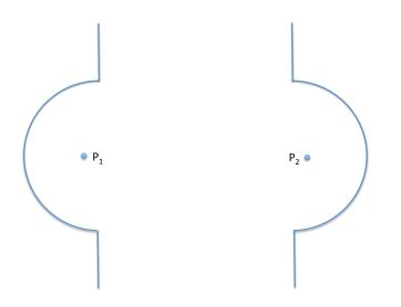
Figure 1: Schematic of the sound mirror. The two people are sitting at the two foci of the mirrors at  $P_1$  and  $P_2$ , talking to each other while facing the mirrors, can hear each other across a crowded, noisy room.
