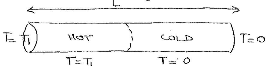
The side walls are insulated so that heat can only be transferred laterally (x-direction).
