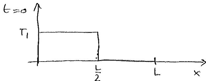
The edges are kept at temperatures 0 and T<sub>1</sub>, respectively.
