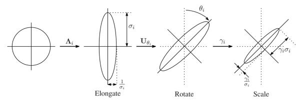
Fig. 9. Schematic representation illustrating the effects of the steering matrix and its component  $(\mathbf{C}_i = \gamma_i \mathbf{U}_{\theta_i} \mathbf{\Lambda}_i \mathbf{U}_{\theta_i}^T)$  on the size and shape of the regression kernel.
