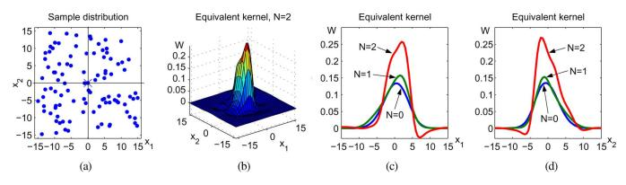
Fig. 6. Equivalent kernels for an irregularly sampled data set shown in (a); (b) is the second-order (N = 2) equivalent kernel. The horizontal and vertical slices of the equivalent kernels of different orders (N = 0, 1, 2) are compared in (c) and (d), respectively. In this example, the kernel  $K_{\rm H}$  in (20) was modeled as a Gaussian, with the smoothing matrix  ${\bf H} = {\rm diag}[10, 10]$ .
