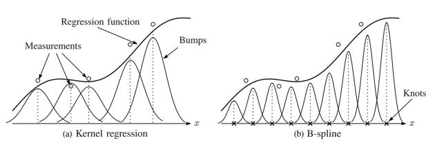
Fig. 4. Comparison of the position of knots in (a) kernel regression and (b) classical B-spline methods.
