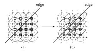
Fig. 8. Kernel spread in a uniformly sampled data set. (a) Kernels in the classic method depend only on the sample density. (b) Data-adapted kernels elongate with respect to the edge.
