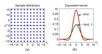
Fig. 5. (a) Uniformly sampled data set. (b) Horizontal slice of the equivalent kernels of orders N = 0, 1, and 2 for the regularly sampled data in (a). The kernel  $K_{\rm H}$  in (20) is modeled as a Gaussian, with the smoothing matrix  ${\rm H} = {\rm diag}[10, 10]$ .
