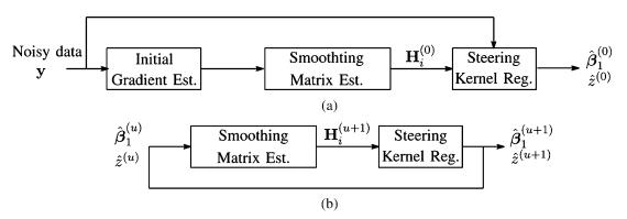
Fig. 10. Block diagram representation of the iterative steering kernel regression. (a) Initialization. (b) Iteration.
