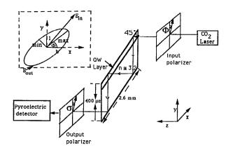
FIG. 1. The propagation of the beam in the 45° bounce scheme. The inset displays the input light, linearly polarized at an angle  $\Phi$ , and the output elliptical polarization.
