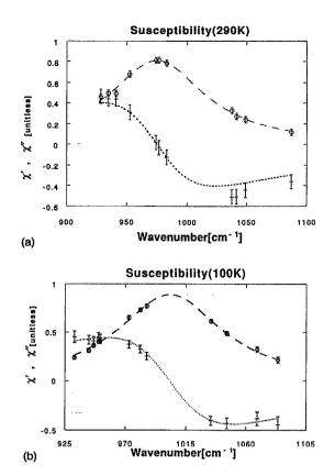
FIG. 2. The measured polarization-dependent real and imaginary components of the susceptibility as a function of wavelength at 290 K (a) and 100 K (b). The dashed line is a Lorentzian fit to the imaginary part of the susceptibility corresponding to the ISBT absorption. The dotted line is a Kramers-Kronig transform of the dashed line—the expected real part of the susceptibility.
