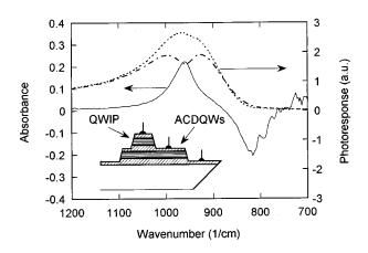
FIG. 2. Absorbance spectrum of the ACDQWs, calculated from the ratio of the photoresponse spectra of the QWIP. Inset: the monolithic integrated device structure.
